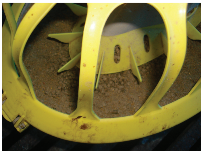
Figure 5: Accumulation of fines in a pan feeder.
