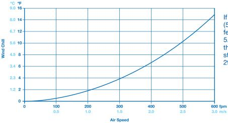
If the air speed is 2.5 m/sec (500 ft/min), the bird would feel approximately 29.4-5.6=23.8°C (85-10=75°F). But the temperature sensor would still show a temperature of 29.4°C (85°F).
