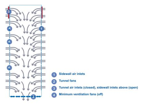
During transitional ventilation, large volumes of air may flow into the house for extended periods of time and birds may therefore feel some air movement on them despite the fact that the operating pressure is correct. Observing bird behavior (the distribution of birds in the house and bird activity) will help to determine how many fans should be operating at a given time. It is particularly important to monitor bird behavior when changing from minimum to transitional ventilation.
