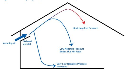
A high air speed will also ensure good mixing of the cold incoming air with the warm in-house air which collects in the apex of the house (**Figure 6.6**). This not only makes the incoming air warmer, but also reduces its RH, allowing it to absorb moisture.
