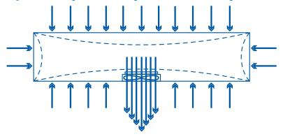
During ventilation, air should enter the broiler house only through the air inlets that are open. The open air inlets must be evenly spaced around the sidewalls of the house. One of the most critical components of a successful ventilation system is how airtight the house itself is. A well-sealed or air-tight house should have no holes, cracks, gaps or any other form of opening, other than the ventilation inlets, through which air can enter the house. This will:
